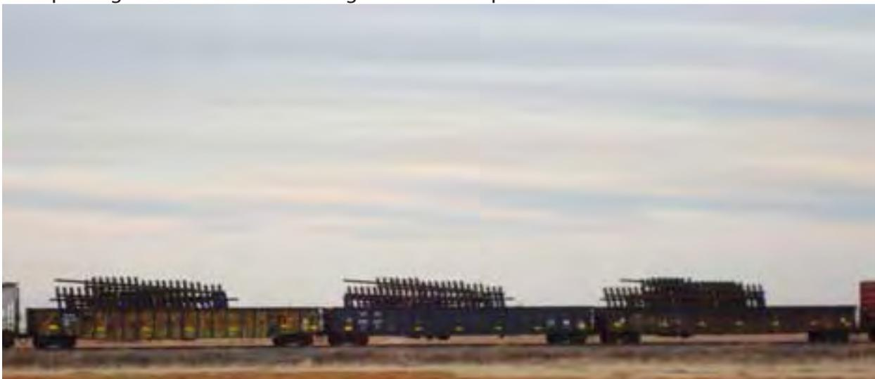
For those of you on the lookout for open loads, here are three condolas with prefabricated turnouts ready for a shoo-fly around a wreck, or for replacement use.
