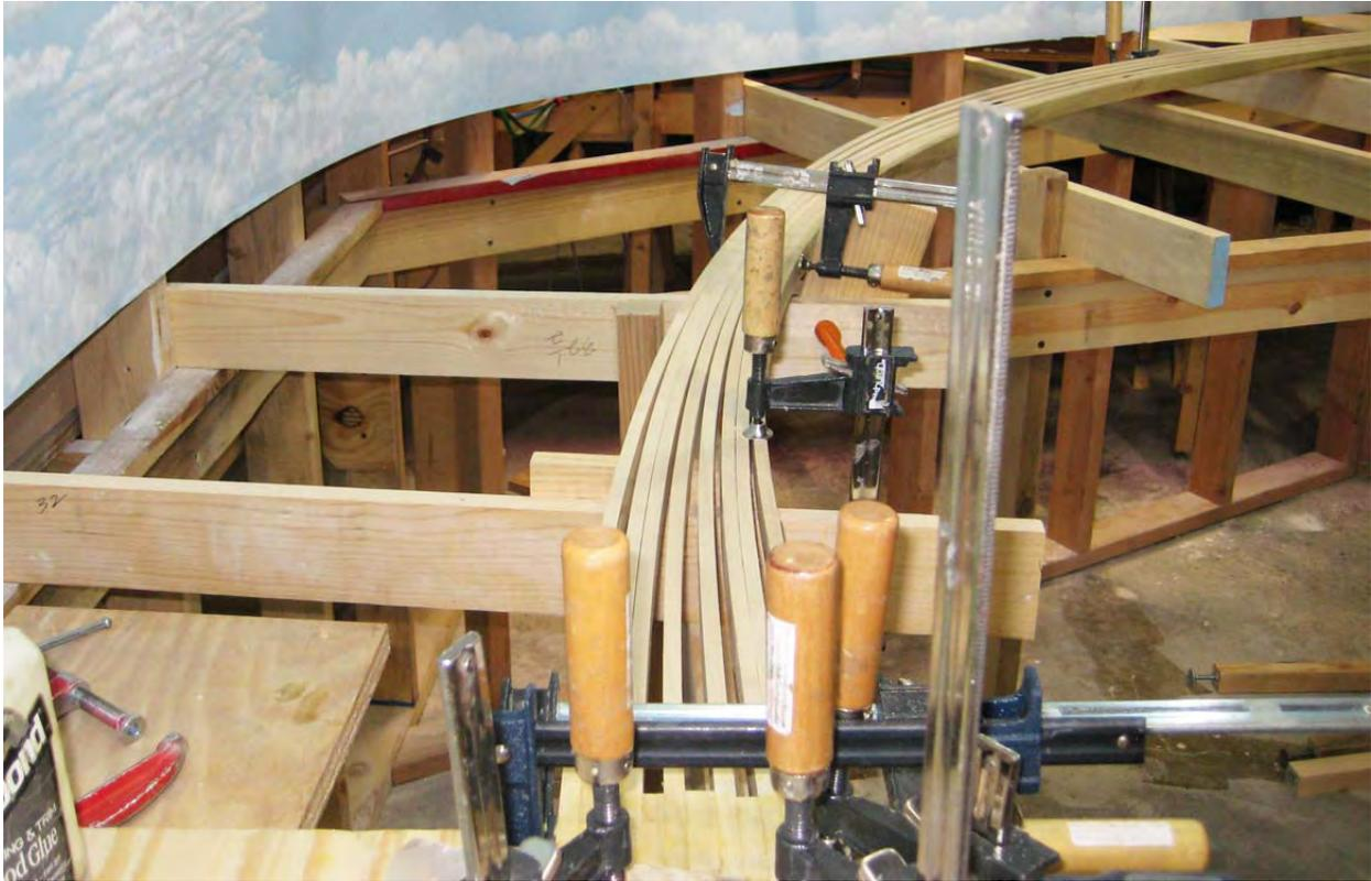
The splines will have spacers between the splines as they take on their final form. This will happen after the glue in the joint is dry. Besides that, the members are tired and hungry and ready to go to Hummers.
