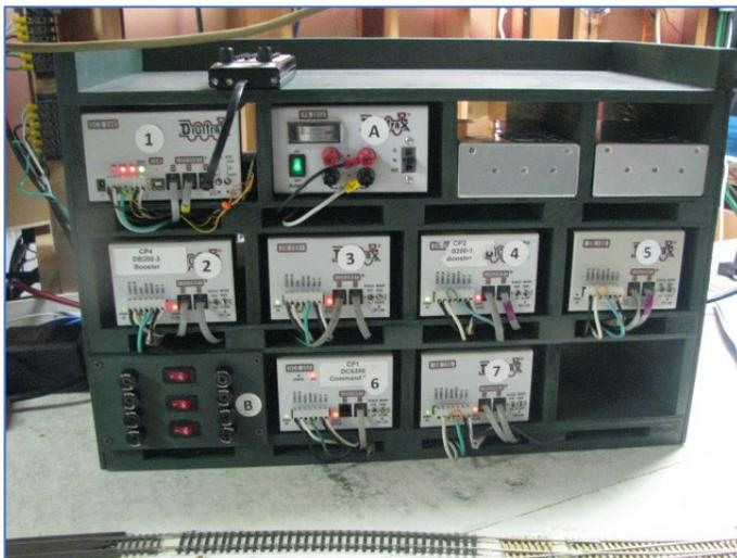
We built a separate 'box' for the power supplies, DCS200 and DB boosters. The power supplies were protected with 8-amp fuses.
