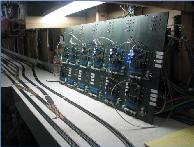
This design became standard for several years. As the layout came along, it was easier to determine the number of blocks we'd need. We left room for expansion if we had to split larger blocks into two or more smaller blocks. In this photo the board is being constructed, with some PM42s not installed. At the time we thought the ability to turn off individual blocks was important, thus the columns of chrome switches.
