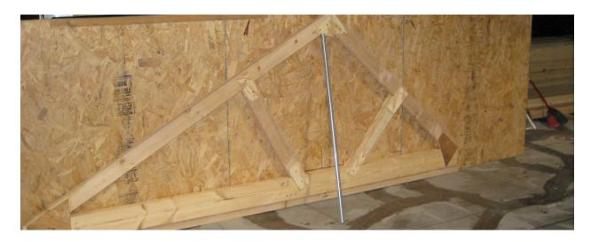
Tracy's Truss Assembly Fixture. We need 50 more just like the one in the fixture
