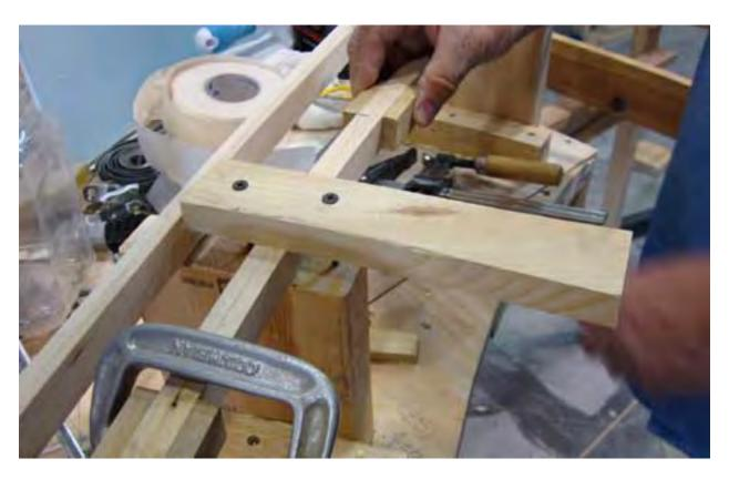
The backbone has been glued. Now the spacer blocks are being glued to the backbone in preparation for the next layer of the spline roadbed.
