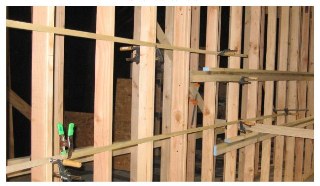
Track level strips coming into Hereford on the upper level and into Panhandle on the lower level. This ewill not be any L-Girders on the upper level. This one is used for study purposes only.
