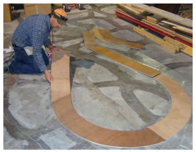
Tracy beginning work on the Canyon Wye, helix and upper level return loop for the upper staging yard. The big circular peice will be split to that the upper half can form a helix passing under itself and entering the return loop.
