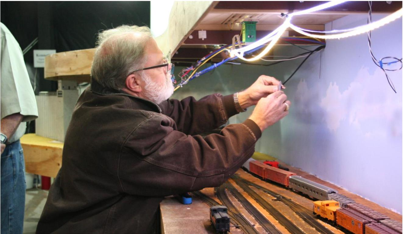
December 12, 2020: Kenneth Berry is preparing to install a connector to the end of the cable to connect to the Tortoise switch machine (see green) for the track on the upper level.
