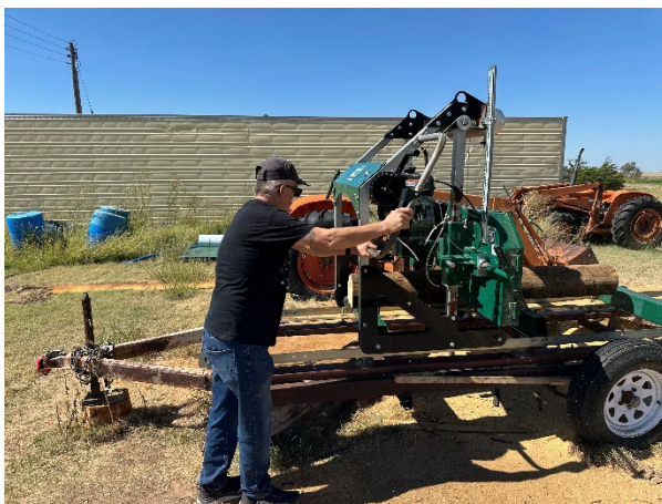
Figure 3 Chris Mitchel working the saw mill to slab logs
